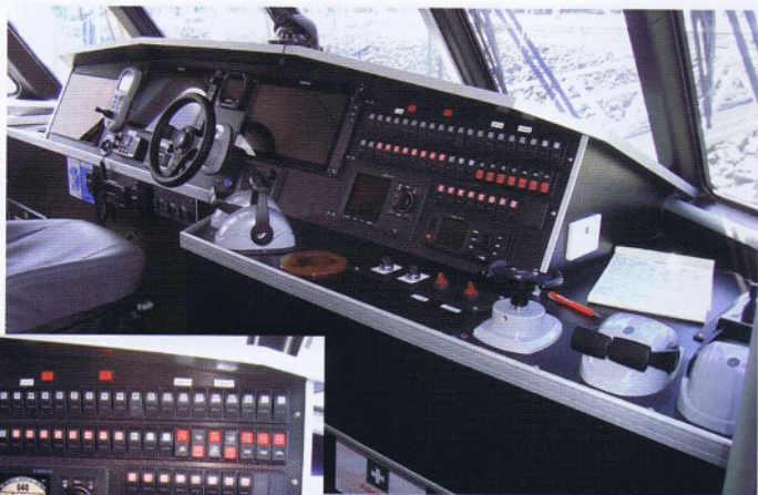
The main conning position with the switch panel close at hand
